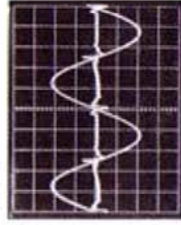
Class B amplifier output waveform and distortion waveform (at 20 kHz)
